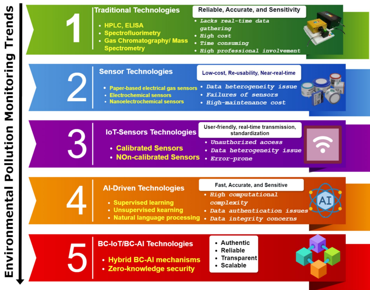
Fig. 4 Trends in environmental pollution monitoring technologies, highlighting the developmental stages and characteristics
