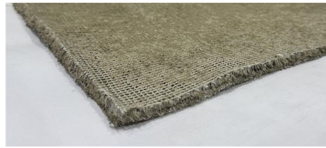
Figure 1. 3D woven textile-reinforced concrete [27].
