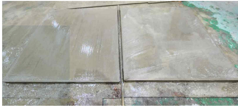
Figure 13. 3D woven textile (SSRM and DSRM) mortar specimen preparation.
