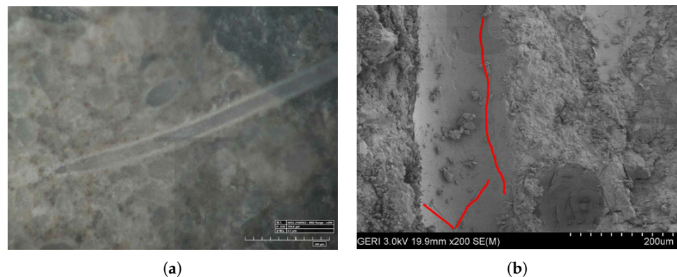
Figure 2. 3D woven textile as observed by optical (a) and scanning electron microscopes (b).
