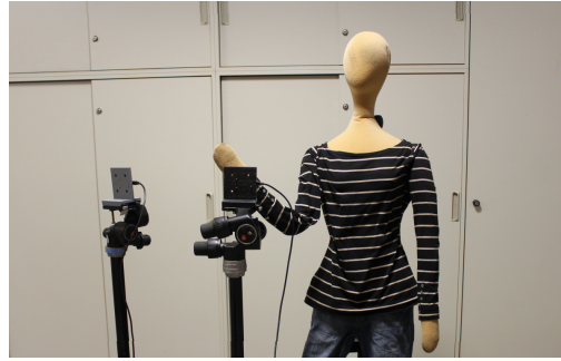
Figure 3. Measurement environment of the KIT radar gesture dataset (Setup 3). This figure shows one representative configuration as an example (reproduced from [36]).
