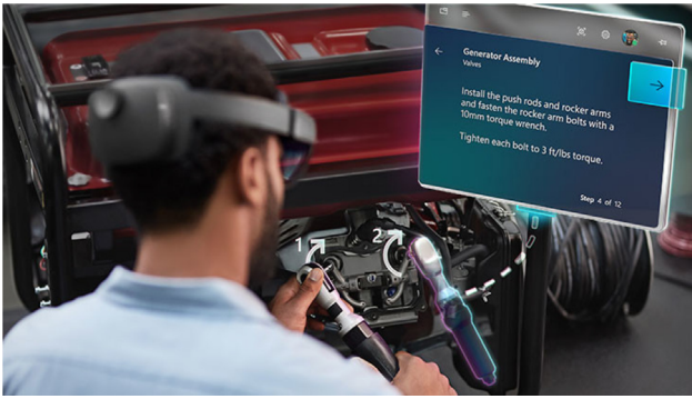
Fig. 9. With the help of Hololens the technician is able to project overlaid step-by-step instructions while carrying out repair on a generator [126,127].
