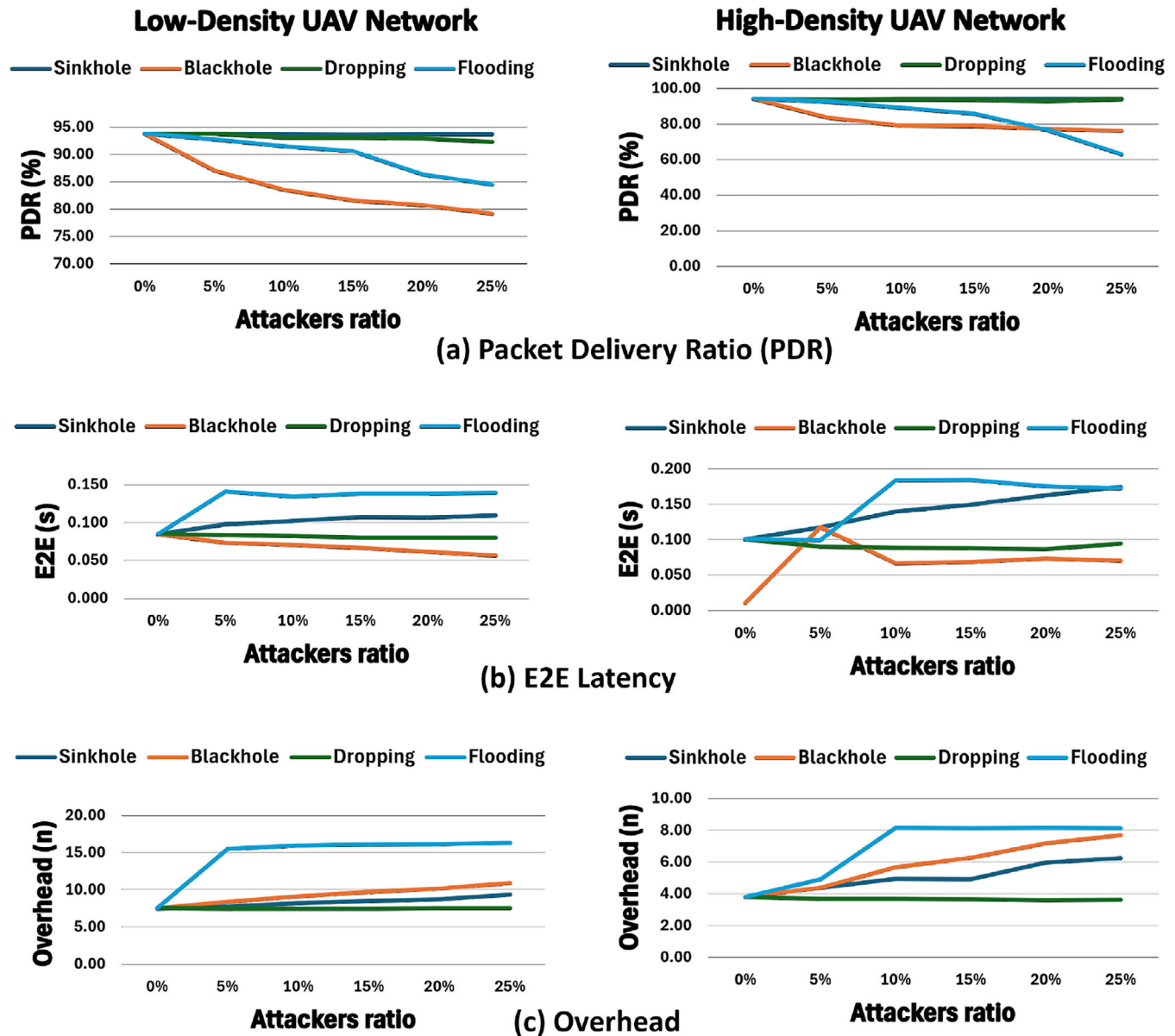
FIGURE 7 Impact of routing attacks on low-density and high-density UAV networks based on (a) packet delivery ratio (PDR), (b) E2E latency, and (c) overhead, with an increase in attack ratio.
