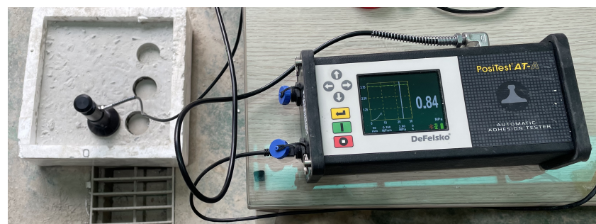
Figure 5. Pull-off testing instrument.
